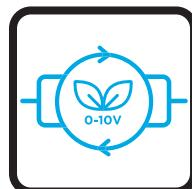
EC motors allow the centrifugal fan to operate at optimum airflow performance, energy efficiency and quiet operation. EC motors include driven control PCB, constant torque, permanent magnet and 3 speeds pre-set or modulating with a 0-10 VDC signal for precise air balancing control. A 5-Speed motor with 3 speeds fixed also available.
