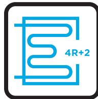
**4 Rows Cooling +2 Row Heating Coil** configurations are available for 4 pipe systems where more heating is required. Other advantages include:
